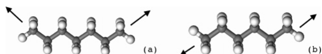
Figure 2. Odd–even effect due to the zigzag shape of the alkyl backbone. (a) The two methyl groups at the end of heptane have a syn conformation, whereas (b) the two methyl groups at the end of hexane have an anti conformation.
